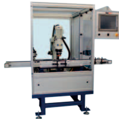
CNC coordinate riveting machine with transfer system for integrating into a transfer line
