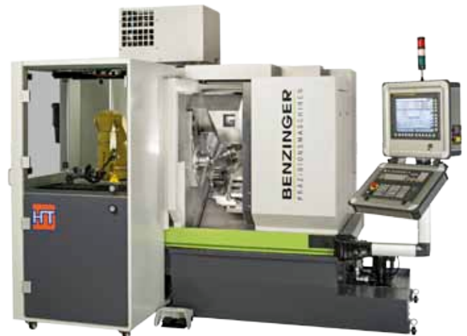
2 work spindles with C-axis, 2 VDI 25 turrets with 12 or 16 tool places, each with a single place drive, Y-axis for both spindles, turret 1 and opposing spindle on separate compound rest, stationary turret 2, simultaneous complete machining
